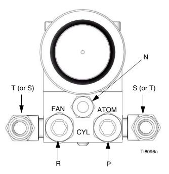
**Bottom Mounted Manifold Ports**
